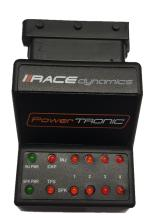
After the completion of installing the PowerTRONIC harness, you can verify the connections are made properly by connecting the stock coupler.
