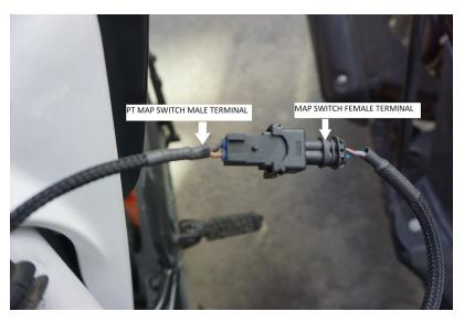
Note: Maps can be changed on the fly. You do not have to turn the engine off to switch between the two on board maps.
